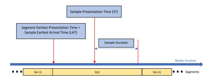
Figure 4 Timing parameters of a timed metadata sample on the media timeline
