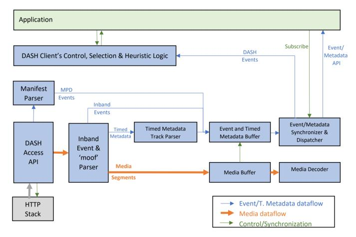
Figure 1 DASH Player architecture including the inband Event and Application-related timed metadata handling
