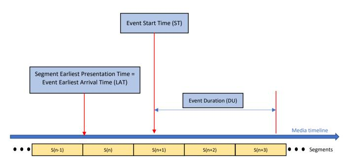
Figure 2 Inband event timing parameter on the media timeline
