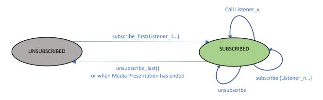
Figure 6 State Diagram of DASH Player for the event/timed metadata API
