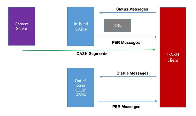
Figure 2 – Assumed system architecture for SAND workflows
