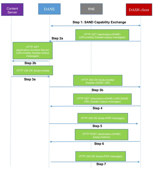
Figure 9 – Example workflow for Consistent QoE/QoS
